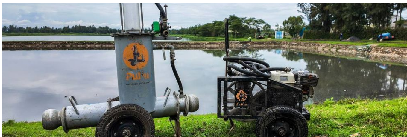
The PuPu Pump at the Nyalenda treatment lagoons. Portable and petrol-powered, it can push sludge up to 70 metres through a hose, which allows a team to work at a distance from the nearest road. PHOTO: OPERO SERVICES, 2026
