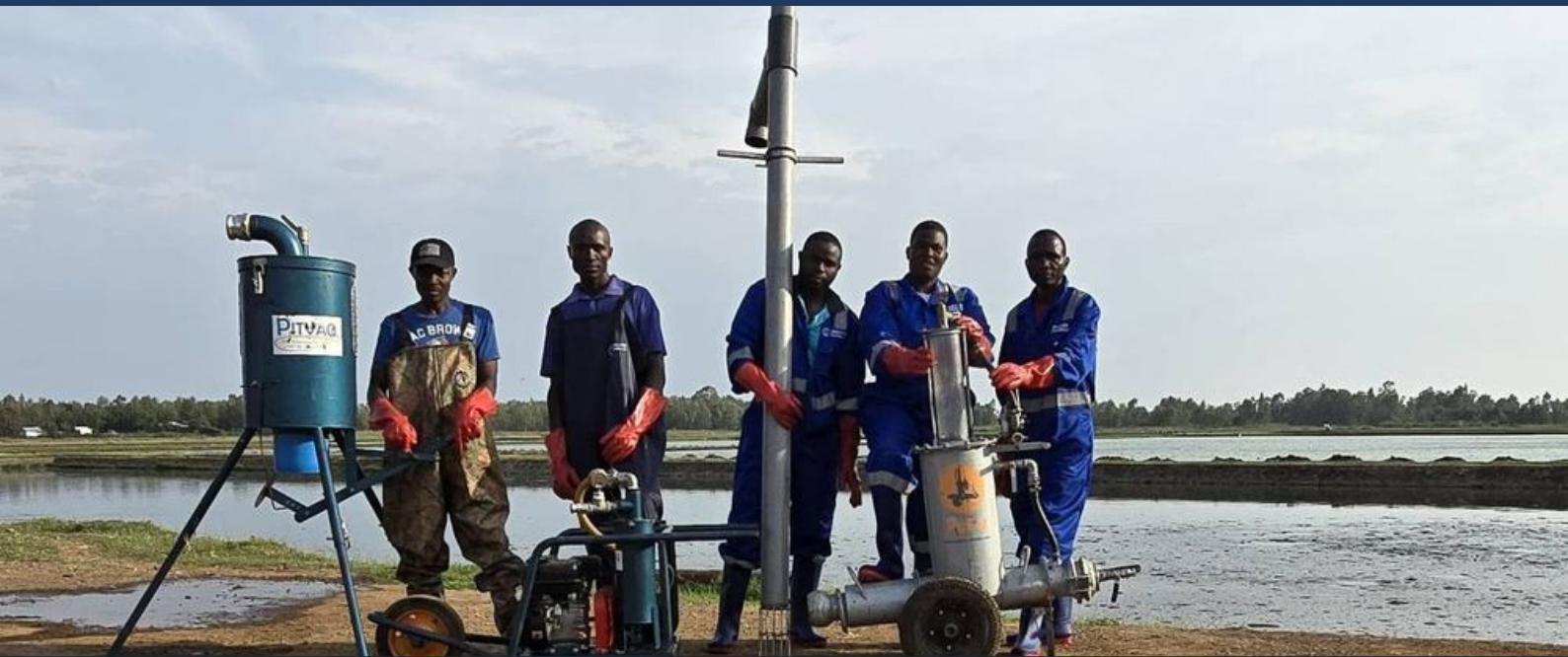
A Kisumu pit emptying team at the Nyalenda treatment lagoons with a PitVaQ, a Gulper and a PuPu Pump.
